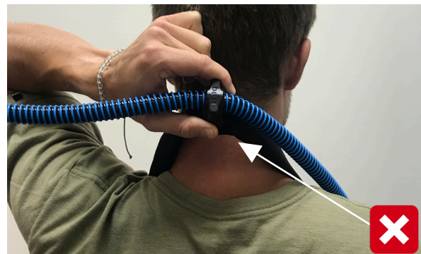
INCORRECT distance of Harness Attachment Point lifting off of neck
