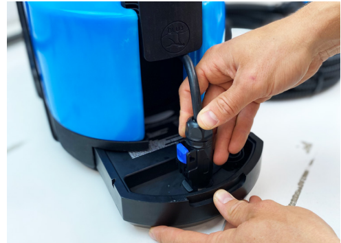
Power cable connector connected to Battery (No. 8)
