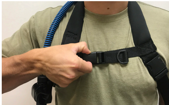
Unclipping the Chest Strap using right hand
