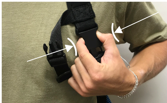
Unclipping the large buckle using left hand
