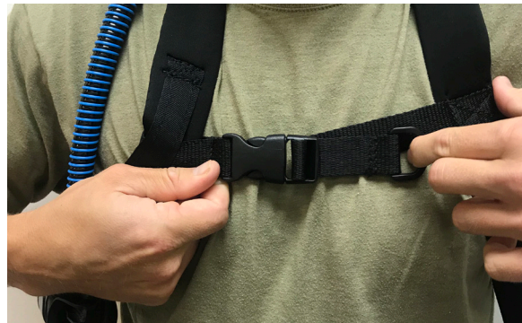
Pulling D-ring to tighten chest strap
