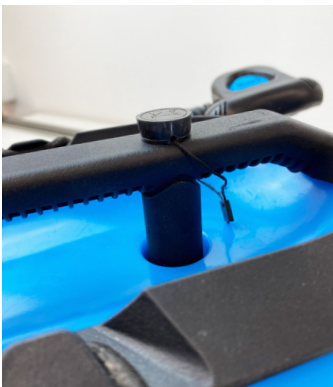
Removal of Intake Plug is Critical for Start-up
