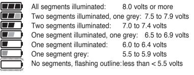
It is recommended to change the batteries when you see one grey segment. If using NiMH rechargeable batteries, the display will remain stuck on the second or third bar for most of the battery life; when it drops to the first bar, the batteries will go dead within minutes.
