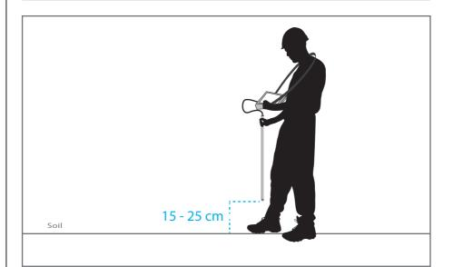
Before starting the user has to balance the device and adjust the sensitivity according to the ground by pressing ENTER or the Button on the top of the Ground Sensor to take a balancing measurement in a stable place unaffected.
