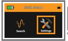
• To set the screen brightness select the icon and press(Enter) to change the brightness from 10% to 100%.
