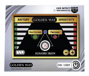
**FERROUS**: if the signal is emanating from non-precious metal, the device will sound in a different tone while the red indicator lights up.
