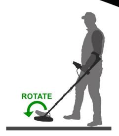
The search coil should be raised almost 2 cm from the ground while keeping it parallel to the ground.
