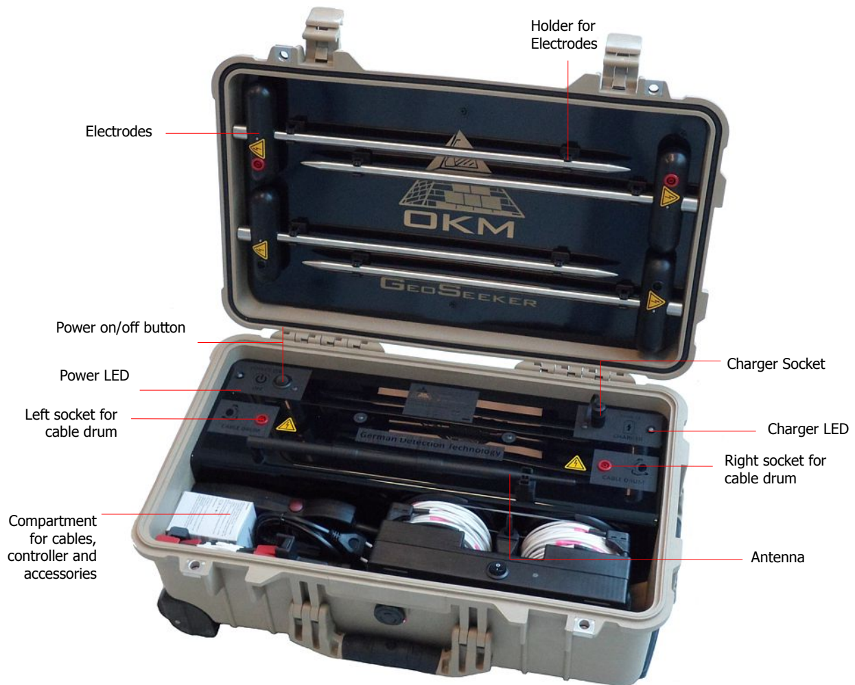
Figure 4.6: Control elements of the Power Box
