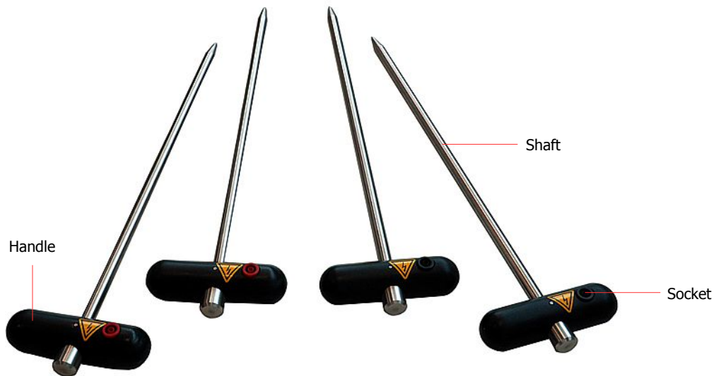
Figure 4.1: Elements of the electrodes
