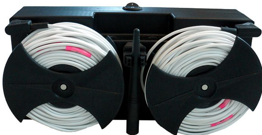
Figure 6.4: Voltage Cable Drums mounted to Controller
