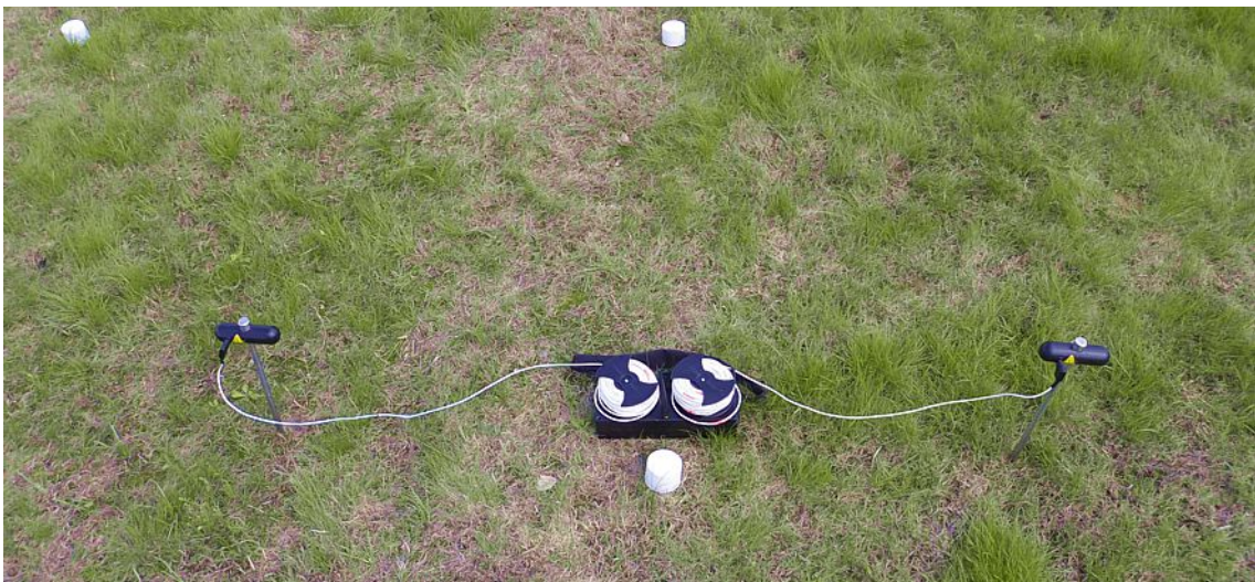
Figure 7.8: Arrangement of electrodes during Passive Scan
