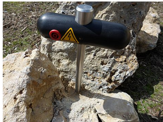
Figure 9.5: Drilling a hole and refilling it for the electrode
