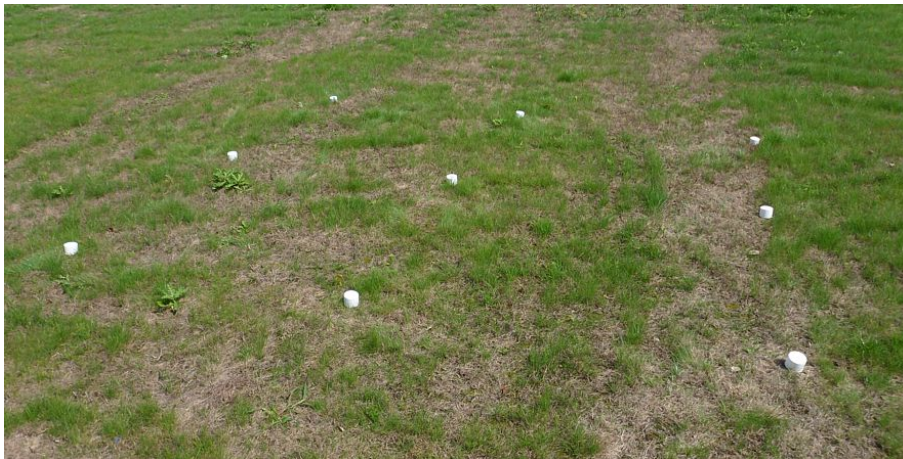
Figure 7.2: Dividing the field into scan points and setting up markers
