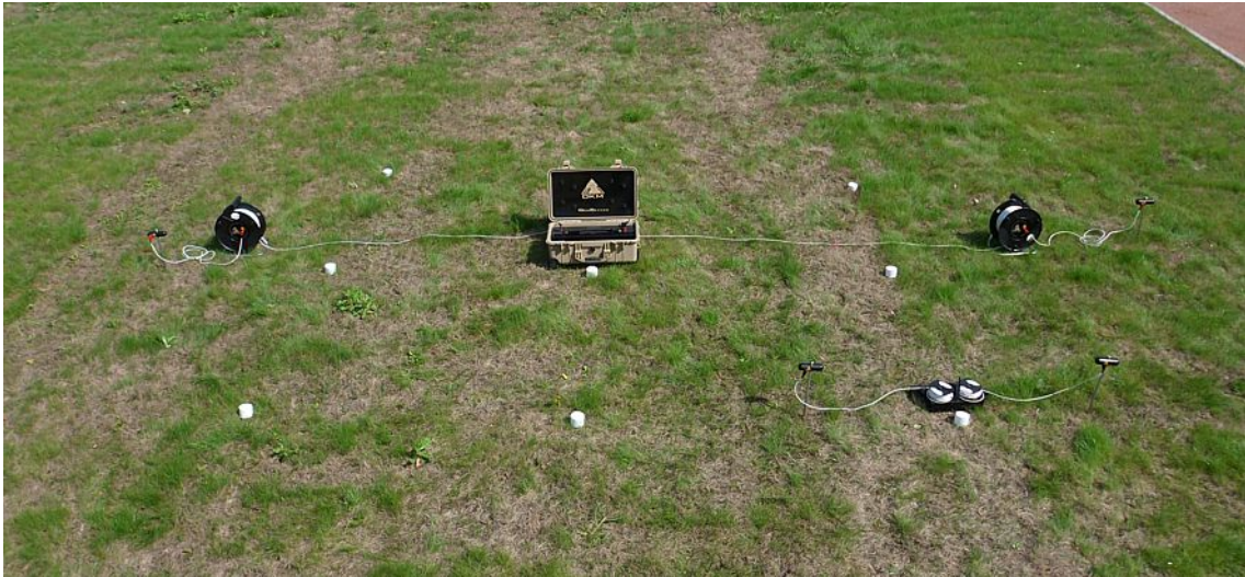
Figure 7.7: Arrangement of electrodes during Active Scan (Quick)
