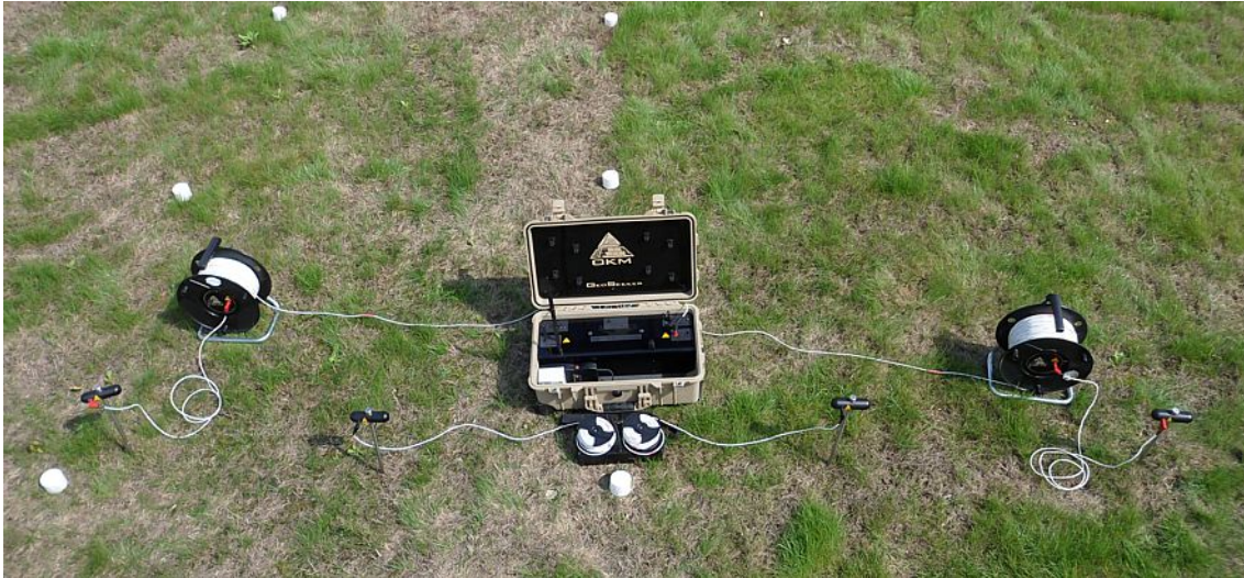
Figure 7.6: Arrangement of electrodes during Active Scan (Accurate)
