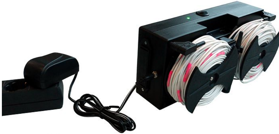
Figure 6.2: Connecting the Controller's charger
