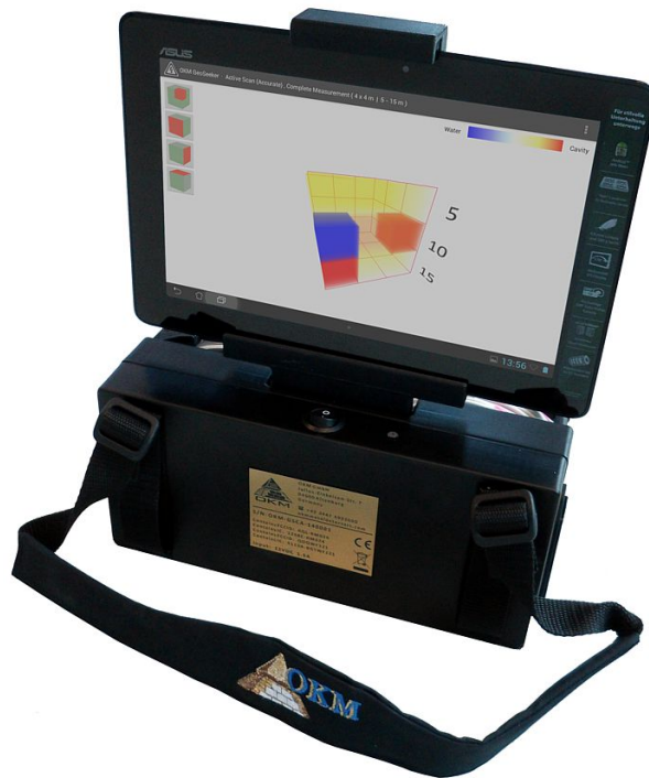
Figure 6.3: Tablet PC mounted to Controller
