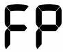
'FP' will appear on the Target ID display when Factory Presets are restored.
