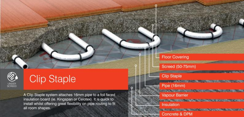
Clip Staple is a very simple and cost effective installation method offering flexibility on pipe routing to suite all room shapes. This system achieves excellent heat output because pipe is laid directly onto a foil covered insulation board and the concrete/screed acts as a conductor and energy store projecting the heat up into the floor covering over a prolonged period.
