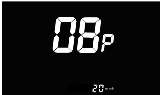
Figure 6-8 Speed limit setting interface
