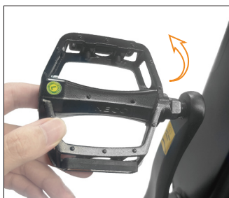
5 Installed on the other side crank.
