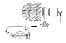
1. Plug the 3.5 mm TRS connector into the audio output jack of your device.
