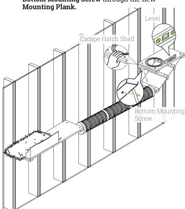
Remove the **18" Escape Hatch**. Install two **Top Mounting Screws** through the **Plank Bracket**.
