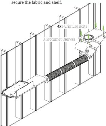
Stretch the 3-Grommet Canvas to the next stud. Line up the Mounting Plank and use the Level to ensure the fabric is flat. Install one Bottom Mounting Screw and two Top Mounting Screws.
