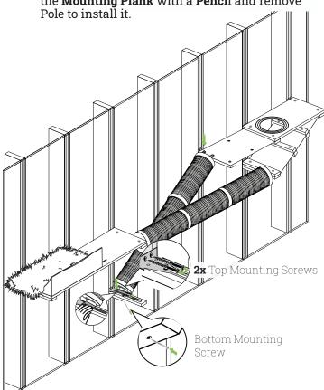
Place a **Plank Top** on each remaining exposed mounting point. Install two **Furniture Bolts** in
