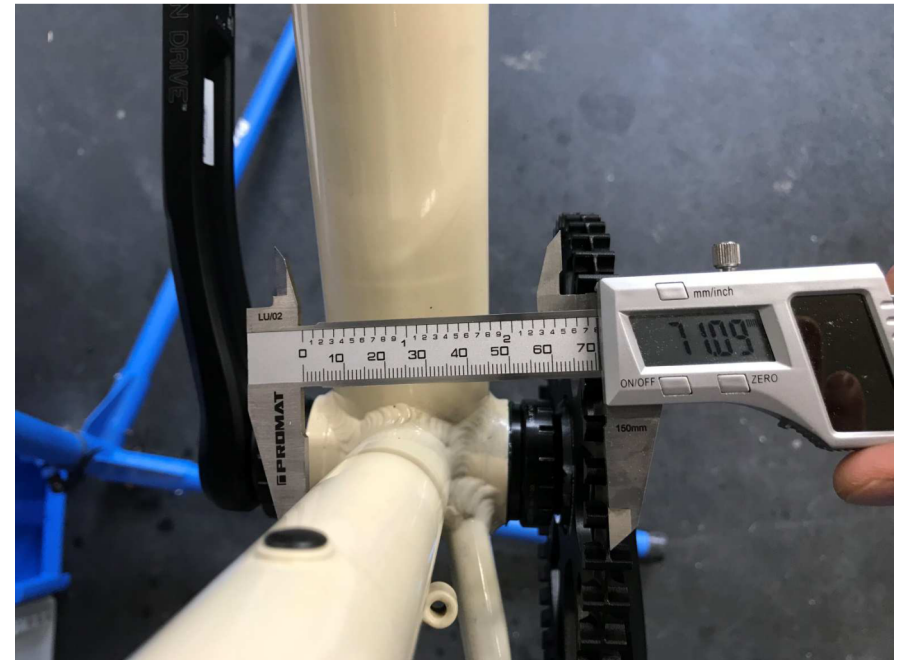
Figure 2: Measurement to center of belt / sprocket
