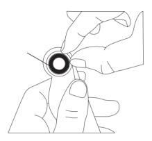
Step 3: Put the spring needle inside the hole of chainsaw.
