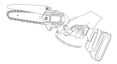
After start, just keep pressing the switch button, you don't need to keep pressing the safety lock.
