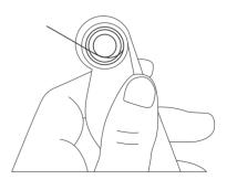
Step 2: Put the screw in the spring.
