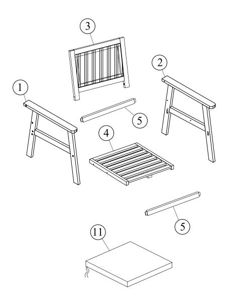
Attach the part 4 to the part 2 using bolt (C) and tighten. Continue to insert the cap (F) and bolt (C) into parts 4 and 2, using the hex key (H) to tighten as shown.
