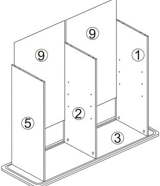
**Step 4:** Insert wooden dowels (C) into parts 1, 2 and 5, as shown. Fix part 4 to parts 1, 2 and 5 with screws (D), as shown.
