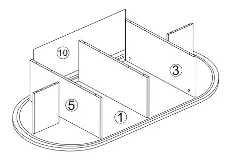
**Step 4:** Insert wooden dowels (C) into parts 3, 4, 5 and 6, as shown. Fix part 2 to parts 3, 4, 5 and 6 with screws (D), as shown.
