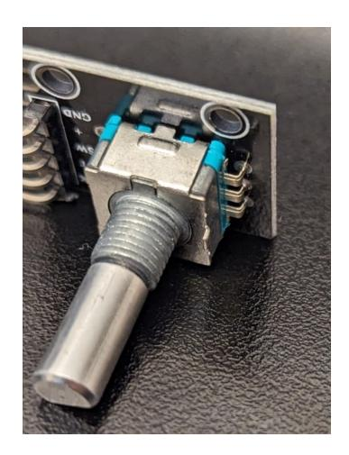
Install the rotary encoder and screw the nut on the exterior side of the Attenuator.
