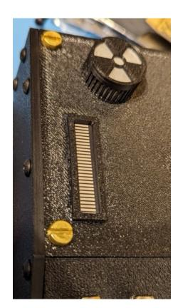
Use CA glue for the radioactive indicator on the shell. Note this is a 2-part piece with the diffuser placed inside the cover.
