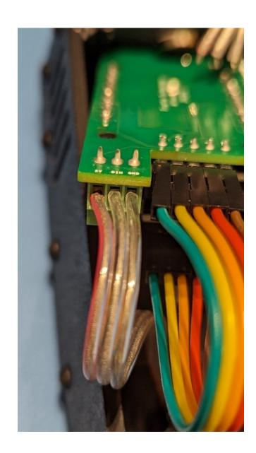
Connect the five coloured cables between the main board and the rotary encoder as shown in the picture. Colours vary, so just make sure the connections on each side are matched up by label.
