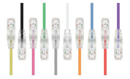
The Ultra Slim Cat6 Cable are constructed of 28 AWG, unshielded, twisted pair, stranded copper with LSZH jacket and high performance RJ45 modular plugs. Space Saving Design - Reduced Diameter: The smaller cable diameter allows twice the amount of cable to be routed through cable managers and pathways compared to traditional Cat6 patch cables. This saves valuable space in a high density environment and at the same time improved air floe and cooling.
