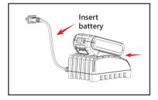
MARNING! Use this charger only to charge the supplied battery or additional purchased batteries that are specifically designed for this tool.
