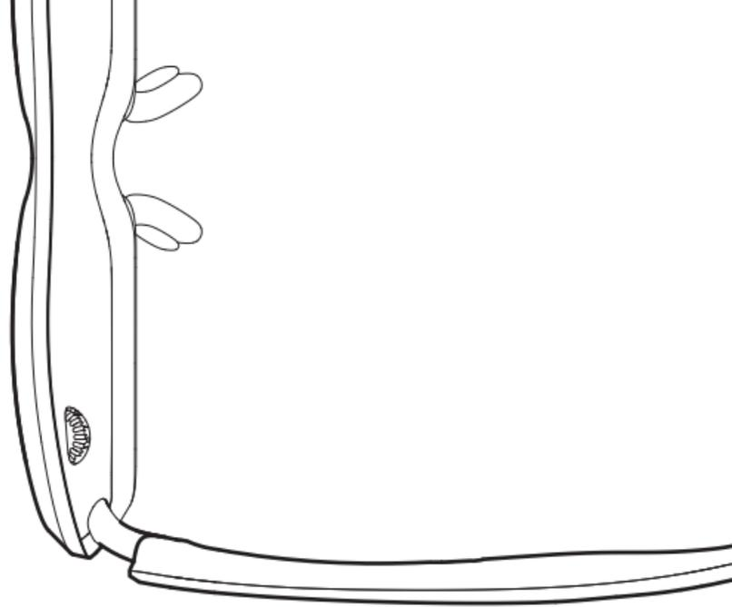
Insert one side of the cable into the USB-C port of the glasses.
