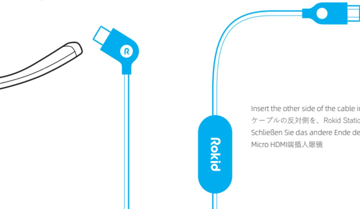
Insert the other side of the cable into the Micro HDMI port of Rokid Station.
