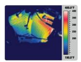
Thermal imaging results with factory synthetic oil
