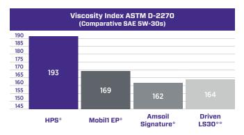
Viscosity Index (VI) indicates the oil's change in viscosity with changing temperature, and is calculated using viscosity measurements at 40C and 100C. Less change in viscosity results in a nigher VI. An oil with a higher viscosity index provides better lubricity and greater protection across all operating temperatures, thickening less when cold and thinning less when hot, \*Information gathered from manufacturers' websites. \*\*Testing performed 2016-2019 by Southwest Research Institute
