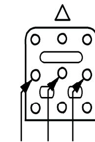
**Connection diagram for 2 speed motors, 2 separate windings, 12 terminals**
