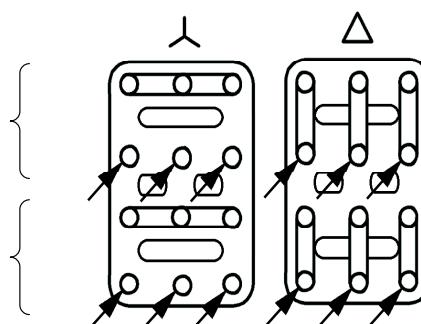
Connection diagram for 2 speed motors, 2 separate winding, 6 terminal
