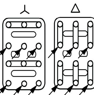
Connection diagram for 2 speed motors, 2 separate winding, 6 terminal
