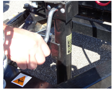
5. Adjust crankstand until crankstand comes into contact with the ground and then turn 1 to 2 revolutions.
