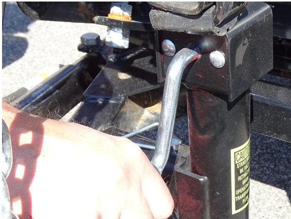
3. Adjust crankstand until it is no longer in contact with the ground.
