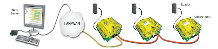
The data line must be wired in a single daisy chain. The data converter may be located anywhere along the data line. 120 ohm terminating resistors must be linked across each data pair at the beginning AND end of the line. This can be done on many units with a switch or jumpers. If not, free resistors are provided with the converter.
