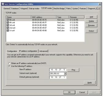
Click on **Detect** and the MAC address of the device(s) will appear in the table. You must then use the "IP address configuration" tab to manually assign the IP address, subnet mask and gateway.
