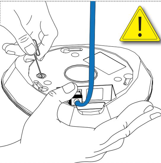
Hold for 5 seconds within 30 seconds of power up.
