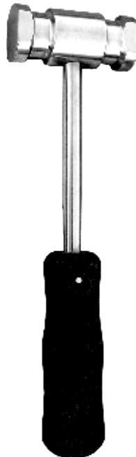
BC318000 Head weight 300 gm Total weight 500 gm 30 mm Ø
