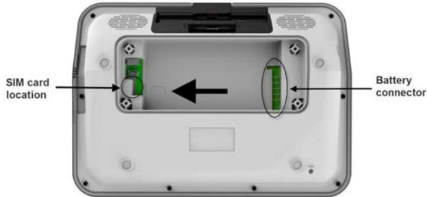
In the battery compartment you will see a small image showing you the correct positioning of the SIM card. Gently slide the SIM card in the direction of the arrow into the SIM card connector.
