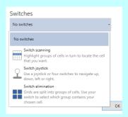
If using a Smartbox switch connector, select Joystick. You can also use a keyboard, mouse or third party device, or even use your entire touch screen as a single switch.
