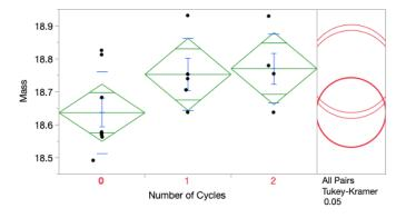
No statistically significant change in mass (0.7% mass increase) was observed. Note that after the initial autoclave, no further water uptake was noted in the second cycle.
