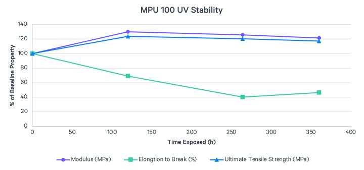
ASTM D4459: Q-Sun XE-1, 0.8 W/m $^2$  at 420 nm, 55 °C ASTM D638: Type V, 500 mm/min, average values represented
