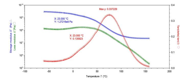
Standard: ASTM D4065 Instrument: TA DMA Q800 DMA Mode: Tension
