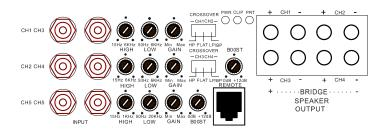
CH1-CH5 RCA's: RCA signal from source
