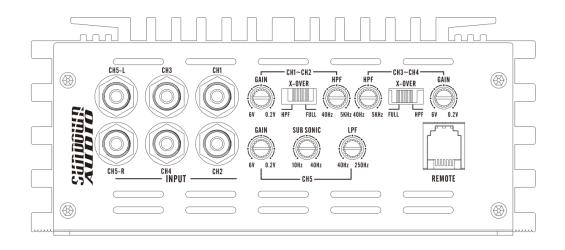
CH1-CH5 RCA's: RCA signal from source
