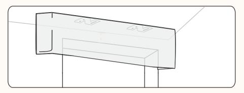
**Installing The Cornice:** After Installing your brackets to the correct width place your cornice over the brackets, center over the window once more.
