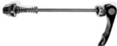
Hub quick-release mechanism CLOSED (Lever at 90° angle to the hub axis)
