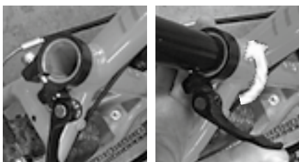
The Figures on the left demonstrate closure of the quick-release mechanism for clamping the saddle.
