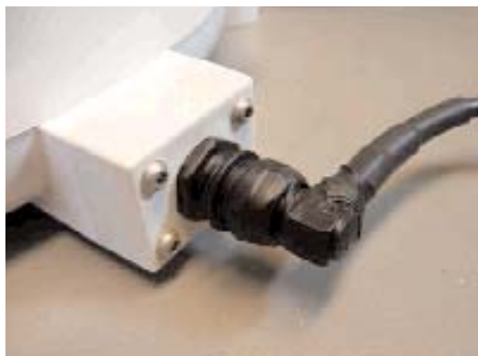
Figure 22 – Antenna Cable Connector Protection
