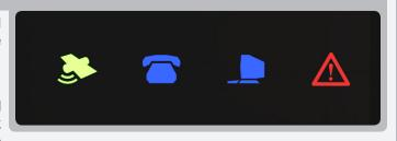
Iridium network. When the Iridium network is found and the ComCenter II successfully registers with it, the satellite icon will stop blinking and stay on solid, indicating the system is ready for use.
