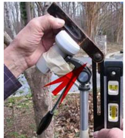
Skews less than 10 degrees CW or CCW don't make much difference, but if you live on the far edge of a satellite beam, skews may approach 30 degrees which is significant. **If your satellite has a built-in offset as in EU's Astra 3B, use the Skew that [www.dishpointer.com](http://www.dishpointer.com) provides.**
