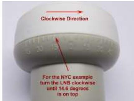
If the reported LNB Skew direction for your location is shown clockwise, you stand behind the LNB looking at the satellite and rotate the LNB clockwise until you arrive at that number. For Washington, DC, you set the skew to 12.1 degrees by turning the LNB in a clockwise direction. Viewing the same satellite on the same longitude, but from South of the equator, result in an opposite rotation skew angle.
