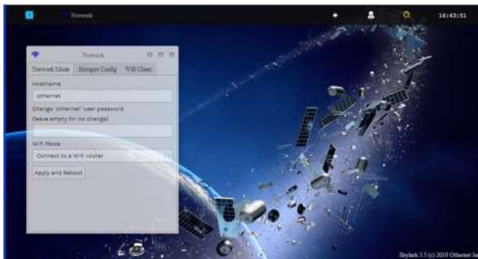
Fig. 25 Network Mode Tab ready to Connect to a WiFi router instead of Create a hotspot Click Apply and Reboot
