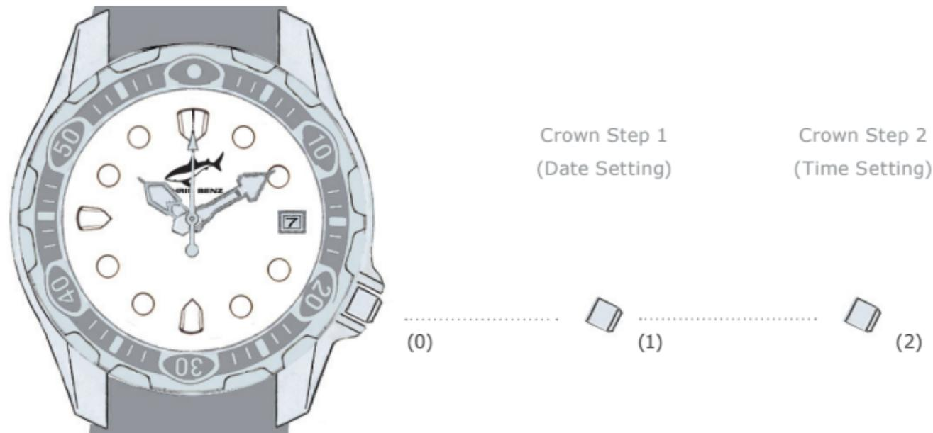
The crown of your CHRIS BENZ DEEP 500M Automatic model is a screw-lock type and has to be opened first before settings can be made! Please don't open the crown in the water or if the watch is wet. The watch will be only water-resistant if the crown is locked and securely closed.
