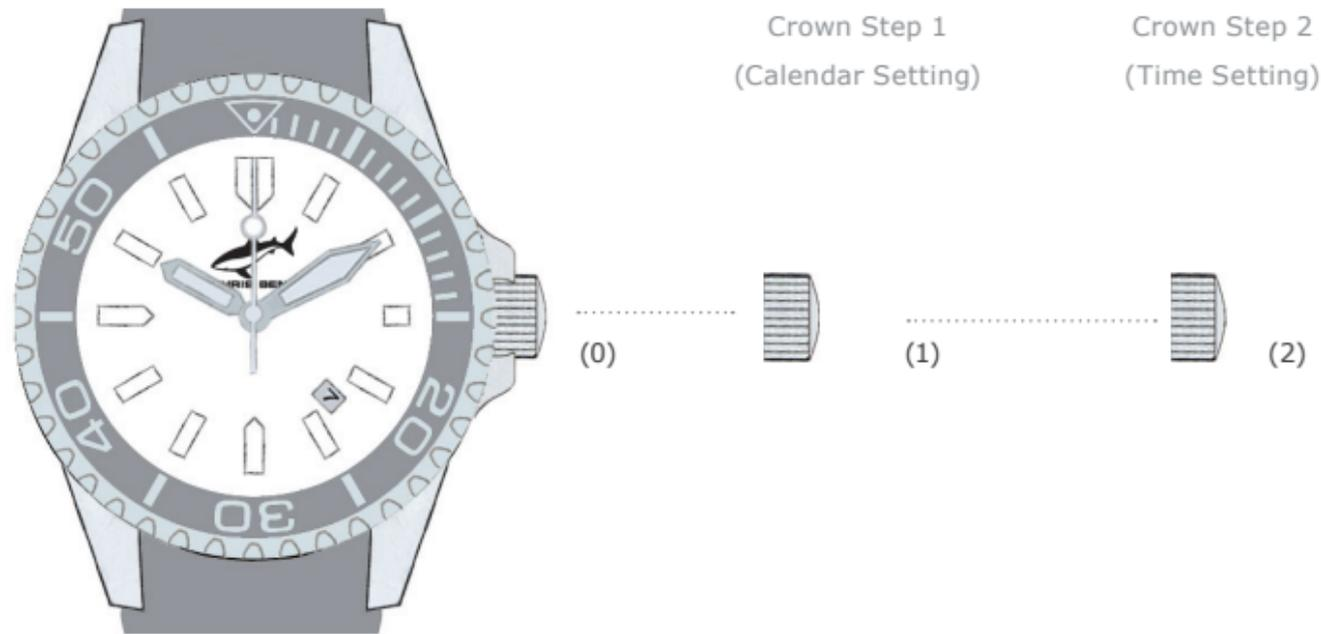
The crown of your CHRIS BENZ DEEP 2000M Automatic model is a screw-lock type and has to be opened first before settings can be made! Please don't open the crown in the water or if the watch is wet. The watch will be only water-resistant if the crown is locked and securely closed.
