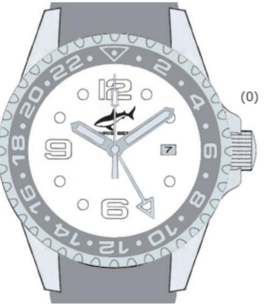
The battery is omitted by the automatic movement. The drivemechanism is powered by the natural motion of the wearer's arm. Without wearing the watch the power reserve will working for up to 36 hours. This may vary however on how long the watch was worn before taken off.
