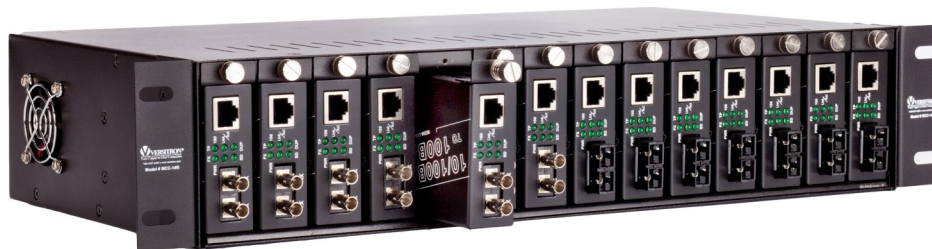
Optional MCC-14R 14-Slot Chassis with Redundant Power
