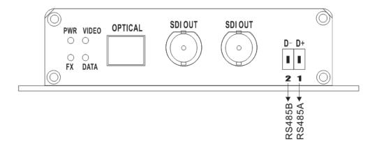
**RS-485 2-Wire Connection (1-Channel Return Direction)**
