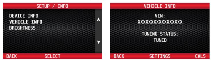
Select 'Settings' to view the current options that are programmed in the vehicle. Select 'Back' button to return to the previous menu. Use the buttons to the right of the screen to view all the settings programmed into the vehicle.
