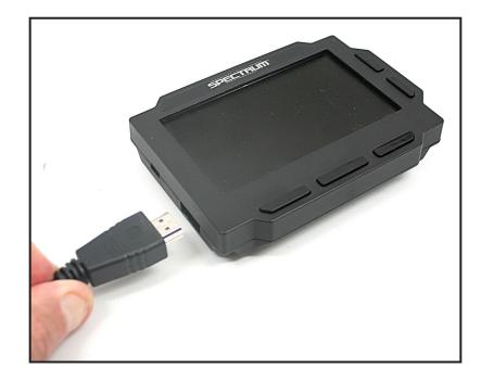
Set the parking brake. Connect one (1) end of the provided cable to the programmer.
