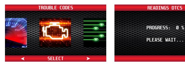
The programmer will immediately begin reading out the DTCs from the vehicle's computer. If no DTCs are present, the programmer will display the following message:
