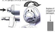
4. Examine check valves if they were removed. Clean as needed. Replace O-rings if damaged. Replace screen if clogged or damaged.
