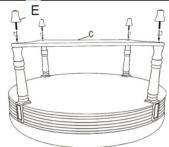
Step1:Insert wooden legs (D) to apron (B) and fasten it by screw with round washer (F/G) by allen wrench (H).
