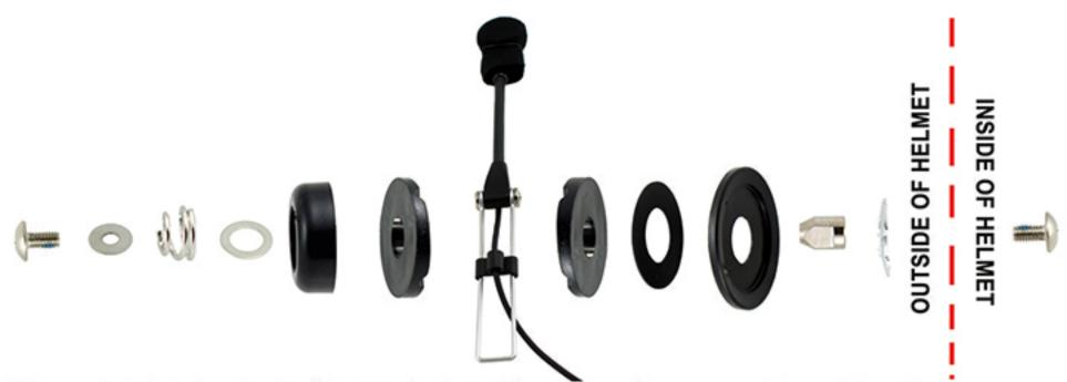
**Step 4:** Tighten both (inside/outside) screws firmly, as this will hold the boom in place and keep it from drooping. Use the smaller phillips screwdriver to tighten the small screw in the wire boom hinge. This will tighten up in/out movement.
