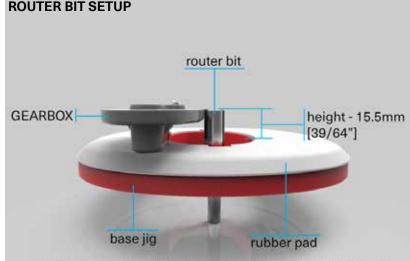
router bit is setup slightly deeper than the distance from the bottom of the box to the top edge off the load beam collar, set the box on the top of the jig as shown to check the distance
