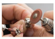
The last polishing stage with rubber polishers is performed with the fine brown polishers 9315F and 9301F.
