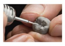
The C31RL, a thin, parallel instrument with special cutting geometry, was developed specially to remove the restoration from the blank. The instrument glides through the material without any tearing and without any build-up of pressure. The extended shaft provides optimised access, even in the case of very thick blanks.
