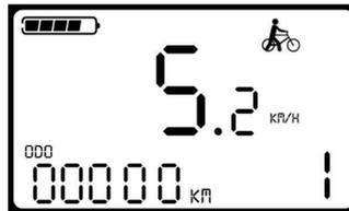
Push-assistance function may only be used when pushing the E-bike. Danger of injury when the wheels of the E-bike do not have ground contact while use the pushassistance function.
